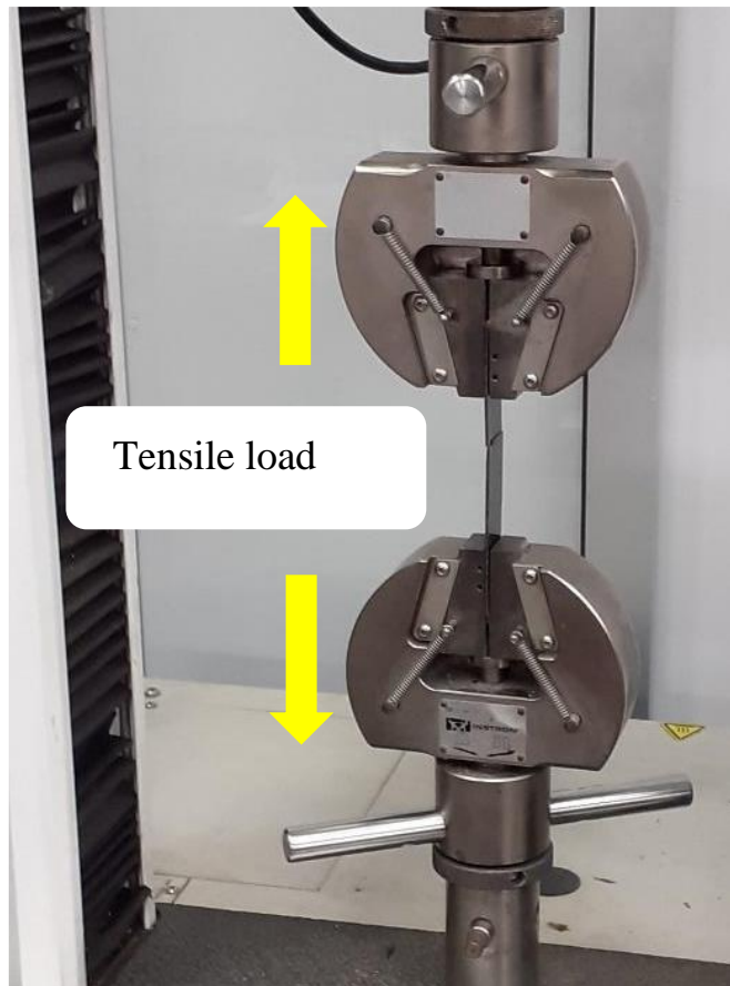
Figure Universal testing machine for tensile testing of Treated SPF/GF/PLA hybrid composite
